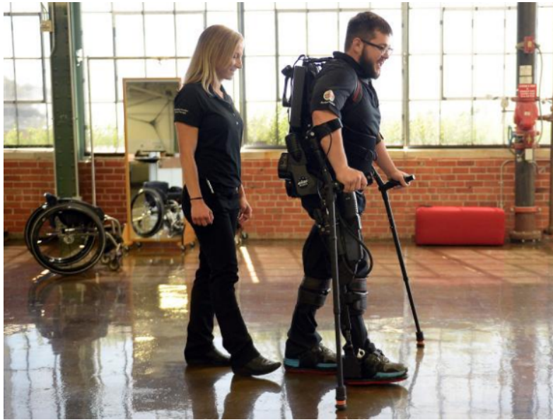
Figure 4.1. Ekso Bionics EksoGT™ lower-limb exoskeleton. The exoskeleton was primarily used for data collection from two sets of sensors: hip and knee encoders. We generated a kinematics-based dynamical model using DSS, and then validated its state-space partitions using foot-mounted pressure sensors at the heel and toe.
