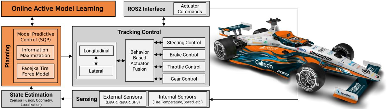
Fig. 1. **Caltech Racer active learning autonomy stack overview.** Our system architecture is comprised of modules for sensing, state estimation, tracking control, and model predictive planning with online model learning tailored for high-speed autonomous racing. In addition to standard state information, the planner estimates tire loads in real-time, which allows it to actively improve model learning.
