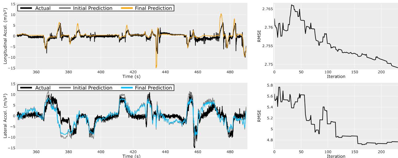
Fig. 4. **Tire parameter identification and predicted vehicle body accelerations.** We show 2.5 min of body acceleration data (left column) from a 30 min run collected during field tests at the Laguna Seca Raceway we fit the parameters of our tire load models. Parameter updates are done in accordance with our specified procedure in batches of 100 samples, resulting in the shown RMSE curves (right column) for the predicted longitudinal and lateral body accelerations.
