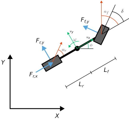
Fig. 2. **Bicycle model.** Diagram of rear-driven bicycle model that lumps front and rear axle dynamics, with forces acting on the car shown in blue.
